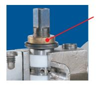
External thrust bearing prevents side loading and extends seal life. No contact with media
