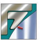
Line contact for lowpressure sealing
